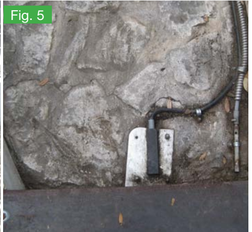
A cleaned inlet with probes
