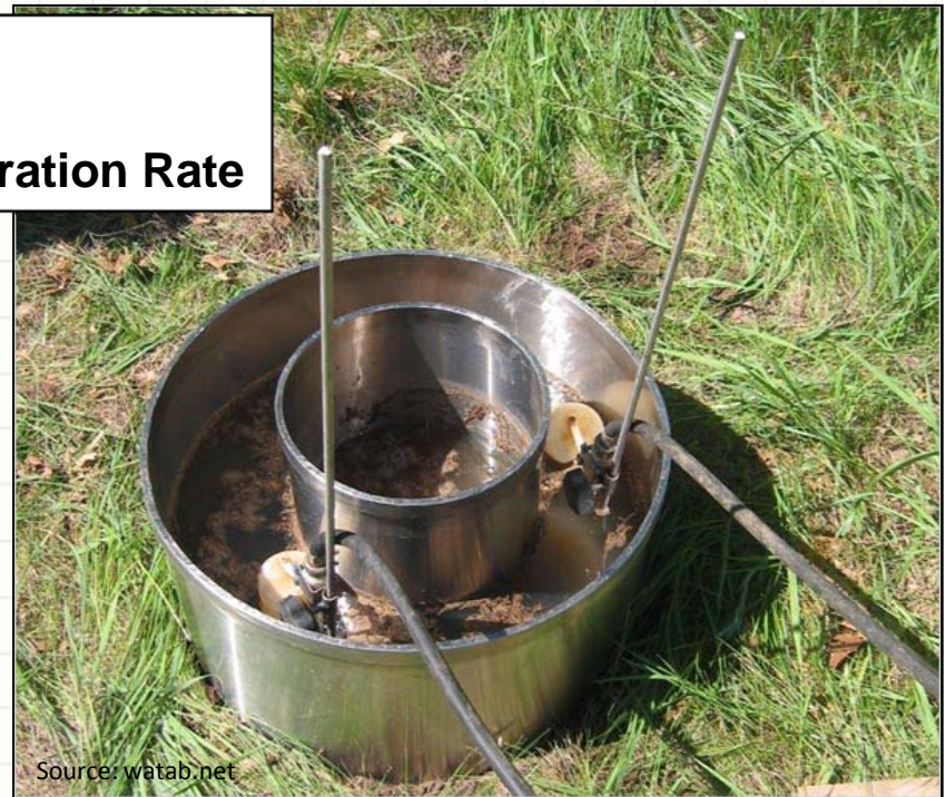
Double ring Infiltration test
