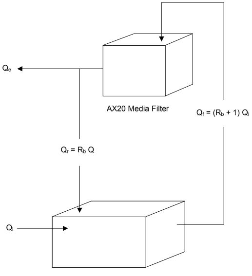
Recirculation/Process Tank AKA Recirc/Blend Tank
