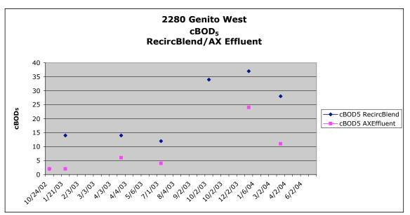
Figure 8: Degradation in Effluent CBOD<sub>5</sub> at 2280 Genito West
