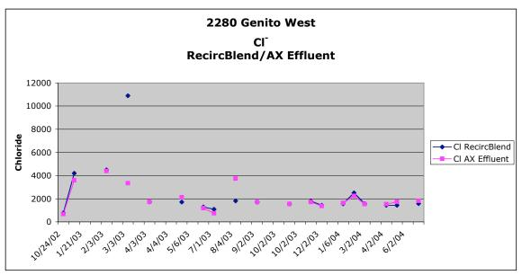
Figure 9: Chloride Concentrations at 2280 Genito West
