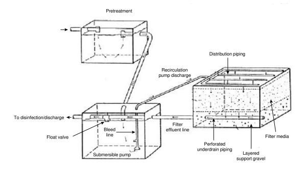
FIGURE 1 TYPICAL RECIRCULATING SAND FILTER
