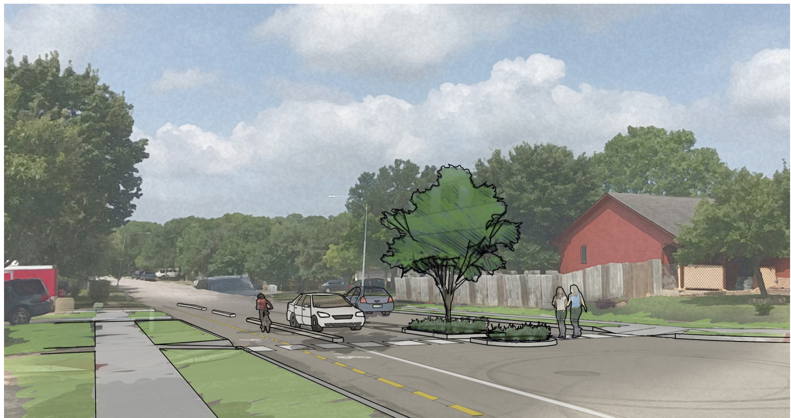
Refuge Island at Siepel Drive and Colony Loop Drive
