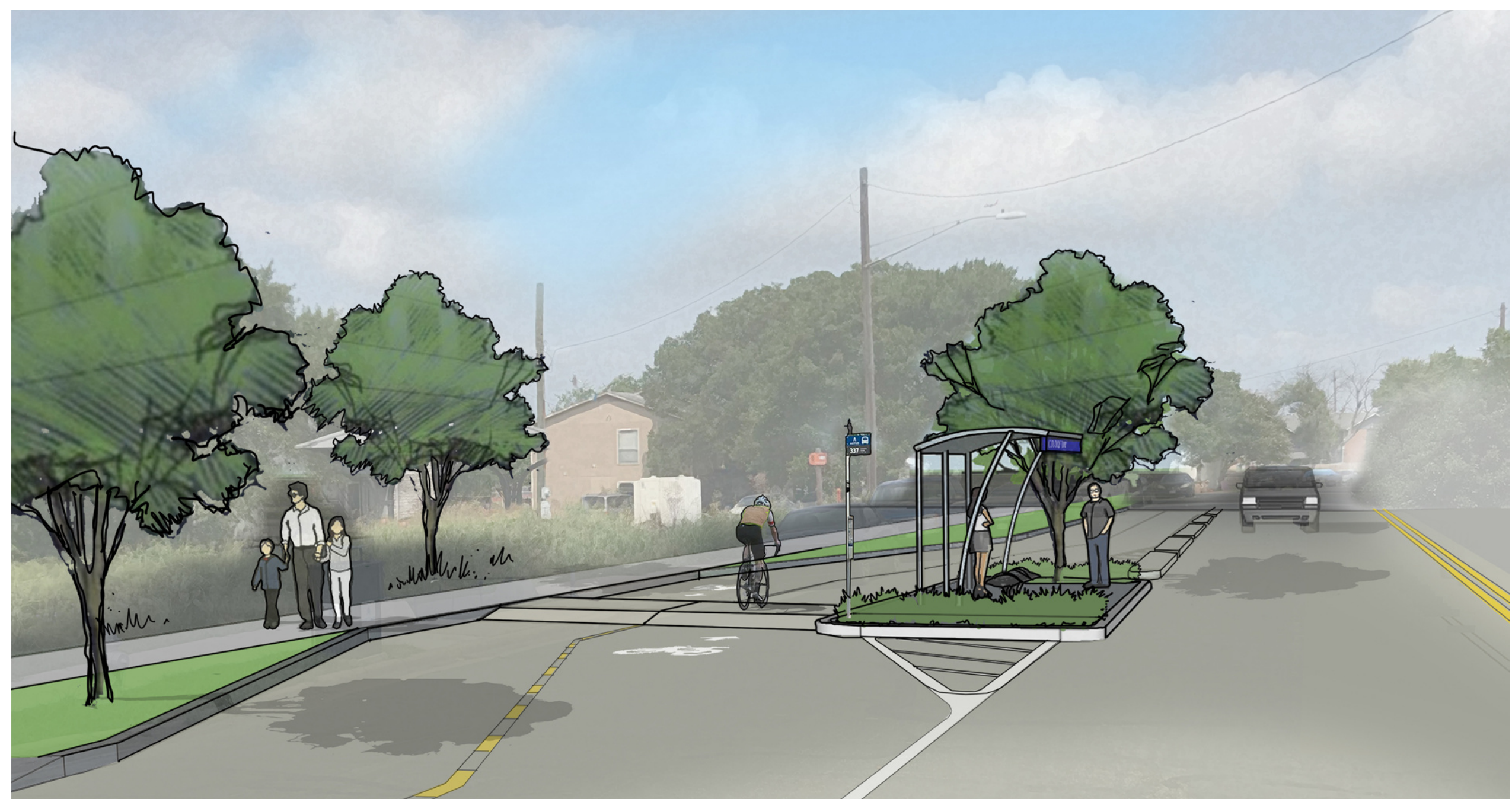
Bus Boarding Island on Decker Lane
